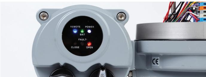
Including a local control station with an HQ actuator provides a quick and easy way to check actuator status and control operation. LCUs, depending on model size/type, offer a variety of controls and displays. LCUs can be as simple as two selector knobs for open/close control, or with indication LEDs, or with a Liquid Crystal Display showing digital valve position.
